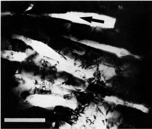
Fig. 2. TEM observation in a foil parallel to the extrusion direction (arrow). Extrusion temperature: 1600°C; scale bar = 2 \mu\text{m} .
